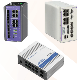
Industrial Ethernet Switches
